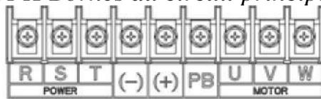
Figure 3-8 : 3PH Bornes du circuit principal (45-110 kW)
